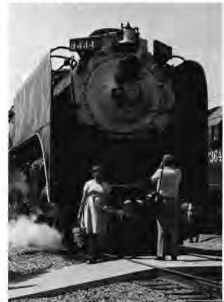
Front view of Union Pacific's No. 8444 a fully operational 4-8-4 built in 1944.
