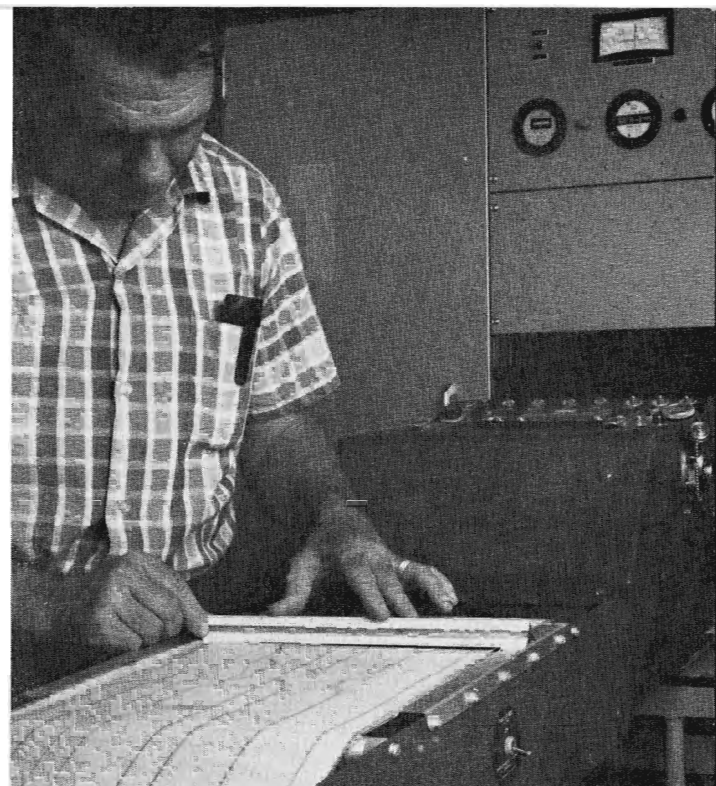
Oscillograph records the fluctuations of tested variables in an instrumentation van beside the tracks. Data on each impact is logged and compared with previous test results.
