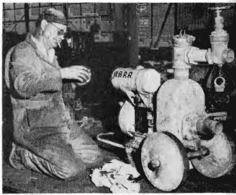
Below: Balser Hefner works on speed prime pump on floor of shop in Oakland.
