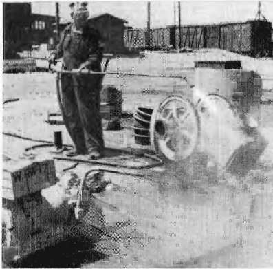
Left: Archie Martin washes equipment with steam and chemicals prior to repair work.
