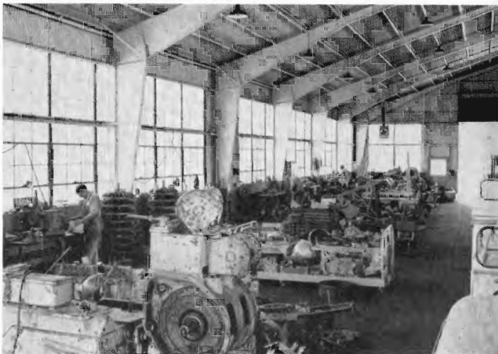
View of shop interior. Shop is well lighted, and equipped with tools for repairing any type of large or small road equipment brought in to the shop for major repair. Minor repairs are done by crews in the field.
