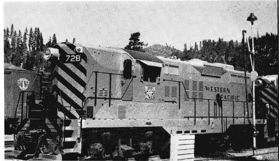
One of WP's newest 1,750-horsepower general purpose (GP-9) single-unit road locomotives delivered recently, and now in service. Eight were purchased at a cost of approximately $1½ million.
