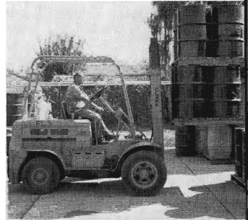
R. V. Wolfe, check clerk, picks up eight oil drums with a 6,000-pound capacity pneumatic-tired yard fork lift truck. Frame overhead is safety measure.
