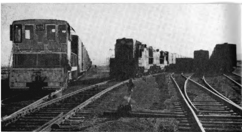
U. S. Gypsum Co. diesel switcher, left, brings in string of loaded cars which will be picked up by Gerlach local's switchers standing by.
