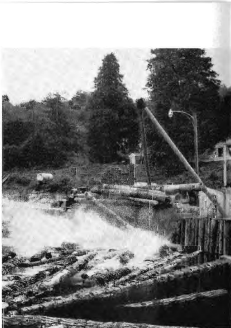
Logs brought down to the mill by truck are dumped into a pond for temporary storage.
