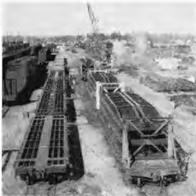
Nearly completed cars wait on assembly line for decking while new frames wait for unloading.
