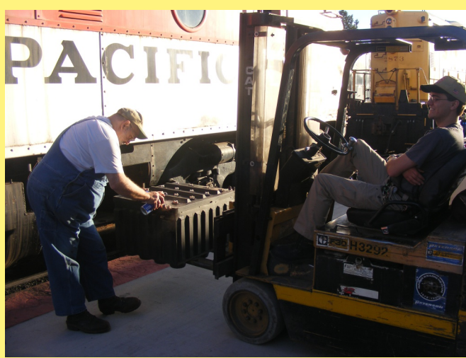
Steve Habeck applies terminal protector after installing the lead connector, while Poindexter waits at the helm of the electric forklift. It's important to remember to use protection.
