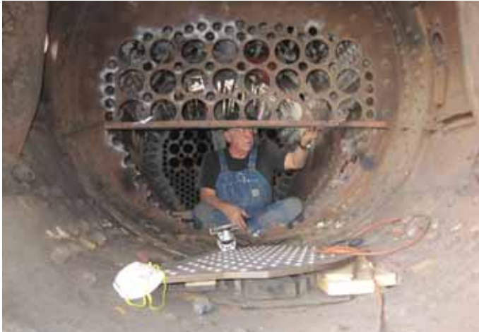
Jim Prettyleaf fitting the new tube sheet.
